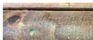
Treatment salts on timber surface.
