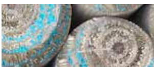
Treatment salts on timber surface.
