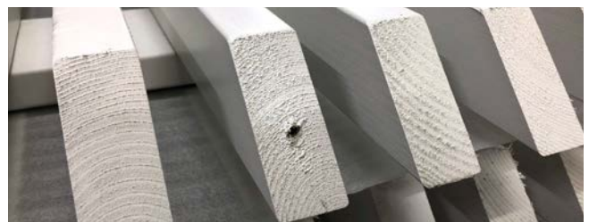
Little holes caused by hanging hooks.
